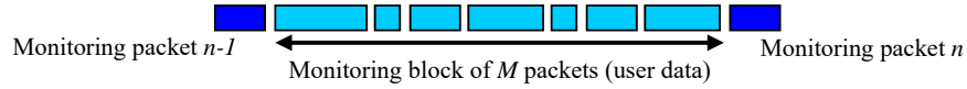
Figure 1: Two monitoring packets enclose a monitoring block that consists of M user packets.
