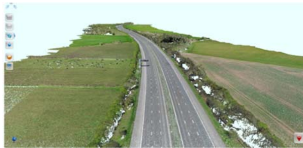
Figure 3: Point cloud Survey with the use of Drones
