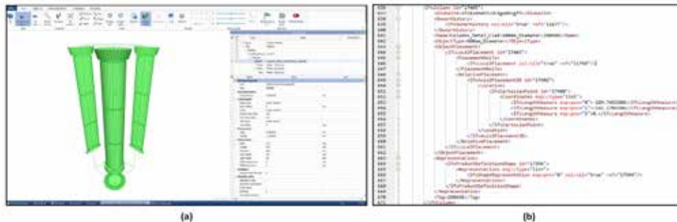
Figure 3: a) The IFC format of a column viewed in open source BIM Vision; b) IFCXML format of the same column.
